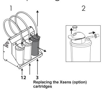
If you purchased an Xsens III set, you can replace an empty can with a full one (A). There must always be 3 cartridges connected.
