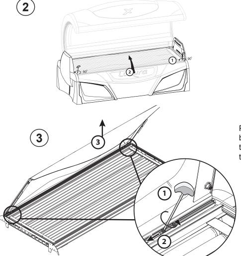
Pull back the acrylic sheet by hand first, and then use the acrylic tool to remove the rest of the sheet.
