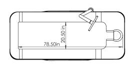
**DISCLAIMER:** A 0.50 KVA BUCKBOOSTER IS REQUIRED IF VOLTAGE IS BELOW 208V OR ABOVE 245V.
